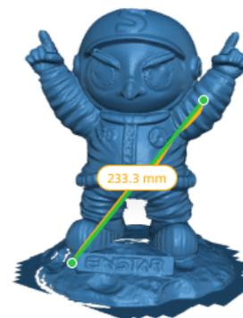
2. After 2 points are added, they will be automatically connected, and the straight line distance (mm) will be displayed; if you add another point, the previous connection will be removed, and a new line will start from the new point.
