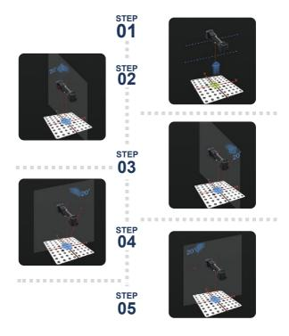
Take the calibration plate out of the bottom of the equipment box, open and place it in a flat position. Pull the scanner farther or closer to the calibration plate according to the instructions of the program until the images at all distances are captured. Move the scanner in pitch and roll to complete the calibration of the scanner.
